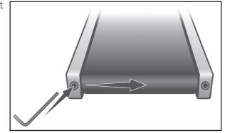
and walking/running characteristics. Some users may affect tracking differently. Expect to make adjustments as required to center the tread-belt. Adjustments will become less of a maintenance concern as the belt is used. Proper belt tracking is an owner responsibility common with all treadmills.
